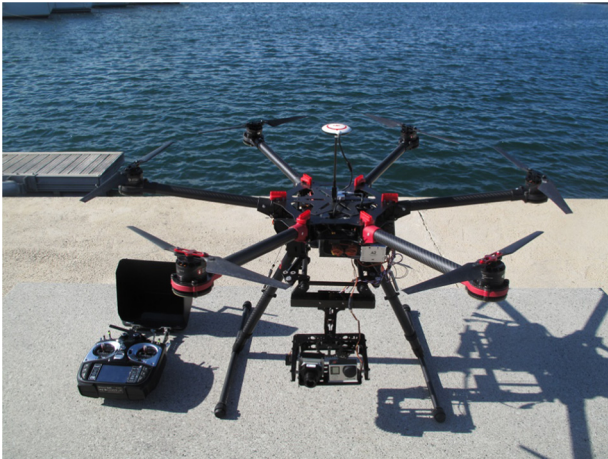
Fig. 5. Hexacopter DJI S900 equipped with a Flir TAU 2 thermographic and a Hero 4 GoPro visual camera. On the left side of the figure is the handheld remote control to pilot the drone and the screen that receives and displays sensor signals.
